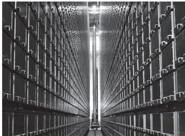
Mansueto Library, University of Chicago READING ROOM ON OPENING DAY (MAY 16); CRANE WITH BOOK BINS
